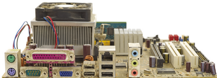
FIGURE 4.4.2 The cooling fan in this computer motherboard circulates air around the electrical components to cool them down.
